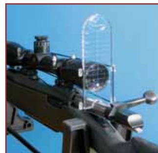
This affordable, easy-to-use lens quickly determines scope alignment problems and makes scope installation faster, easier, and more precise. The engraved lines on the lens allow the scope's vertical crosshair to be plumb with the bore as it squares the horizontal crosshair. When it's plumb, it's level.
