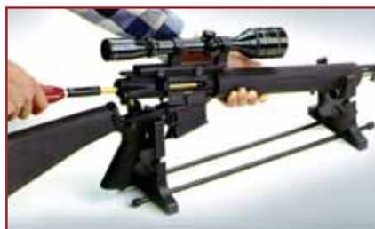
Simply hinge open the upper and lower receivers and remove the bolt and carrier. Install the Bore Guide's tapered nose snugly into the chamber opening as the slide-adjustable collar is positioned in the action. Use the brass pin (with protective tip) to lock the Bore Guide in place and to hold the upper and lower receivers at a proper angle. Commence cleaning, with the same benefits as with bolt-action rifles!
